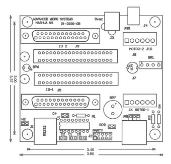
An RS-232 input converts standard serial voltages to TTL levels to drive up to 10 axis using Advanced Micro System's "Party Line" protocol. The open drain TXD outputs from each axis are wire-or'd, providing a party line communication method. Prior to operation each axis must be assigned a one character name that is stored in the CCB-26 NV memory. Removing the "Party Line" jumper and inserting one axis at a time facilitates name assignment.
