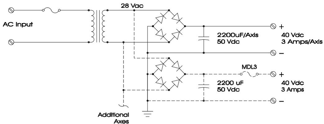
If multiple drivers are used with one power supply, each drive should have separate power and ground wires that connect directly to the output capacitor of the power supply.
