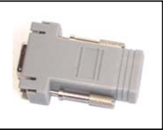
Passive serial adapter. Connects RS-232 (DB9) to IBC-400 serial input. No intelligence – use for single axis only. Includes 7 foot cable. Model: SIN-9
