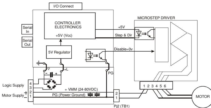
The logic “controller” section consists of microprocessors, a logic encoder and analog processing.
