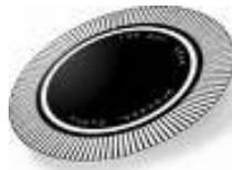
The more common encoder is the incremental design. An incremental encoder produces a series of square waves as it rotates. The number of square wave cycles produced per one turn of the shaft is called the encoder resolution.
