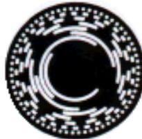
Absolute encoders output a unique digital numeric for any given position of the encoder's rotation. They are used in applications where a device is inactive for long periods of time or moves at a slow rate, such as flood gate control, telescopes, cranes, valves, etc.
