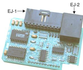
EJ-1 is a 12 contact signal connector (Molex SL Crimp series). EJ-2 is an 8 contact RJ45 encoder input connector.
