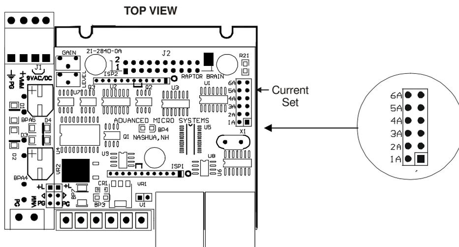
*Note: Damage to the motor can occur if the driver setting exceeds the motor rating.*
