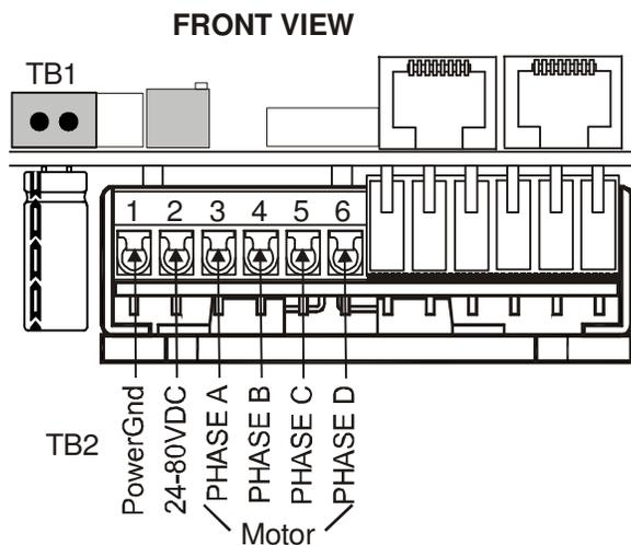
**CAUTION! Damage to the mSTEP-407 will occur if the motor leads are shorted to each other or to ground and/or the motor is plugged or unplugged when power is applied.**
