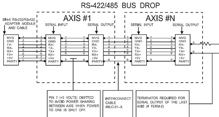
**Note: Pin 8- Party is not used in products utilizing the ^N and ^P commands.**
