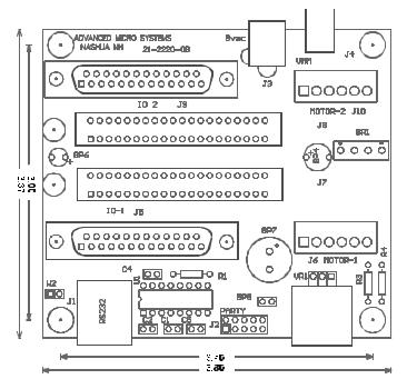
An RS-232 input converts standard serial voltages to TTL levels to drive up to 10 axis using Advanced Micro System's party line protocol. The open drain TXD outputs from each axis are wire-or'd, providing a party line communication method. Prior to operation each axis must be assigned aone character name that is stored in the CCB-25 NV memory. Removing the "party" jumper and inserting one axis at a time facilitates name assignment.
